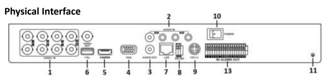
\*: The rear panel of DS-7204/7216HUHI-K2 provides 4/16 video input interfaces.
